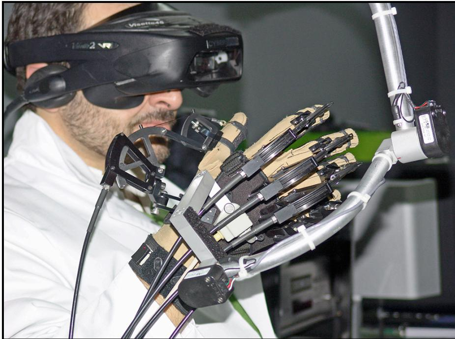
**Fig. 3 - A view of the visual-haptic delivery simulator test-bed, featuring an Immersion CyberForce hand-based haptic device.**
