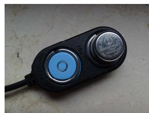
Fig.2 – iButton Datalogger
