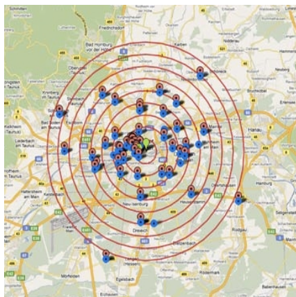
Fig.1 – Neighborhood of a vehicle (green marker). Blue markers indicate actually existing nodes and red markers indicate discovered nodes.
